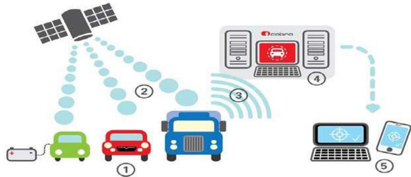
The Cobra Telematics solution in the vehicle (1), obtains vehicle trip data and also GPS position (2), which are transmitted via GSM/GPRS/3G (3), to the server at the Cobra Service Centre (4), from where they are made available to the customer via phone or internet (5).
